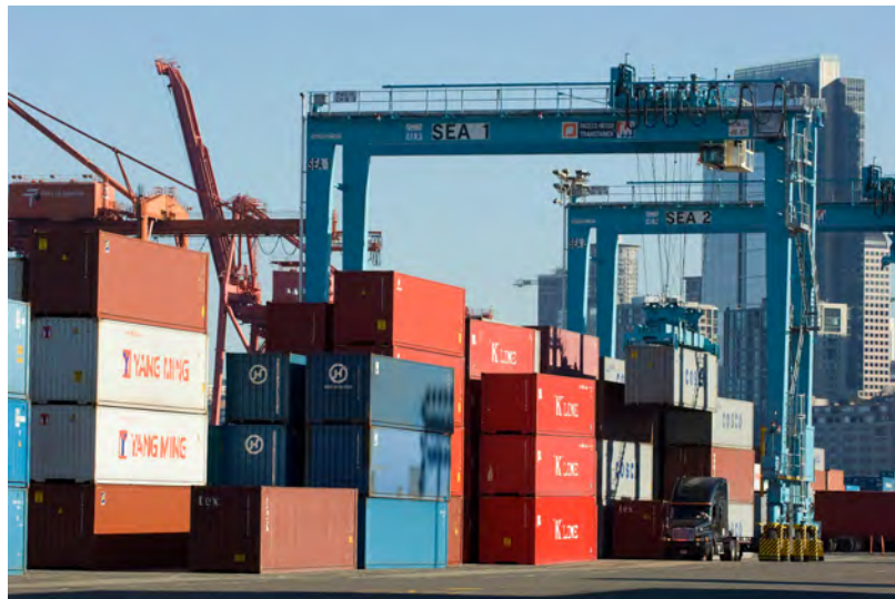
Figure 5.4: Rubber Tired Gantry Crane
