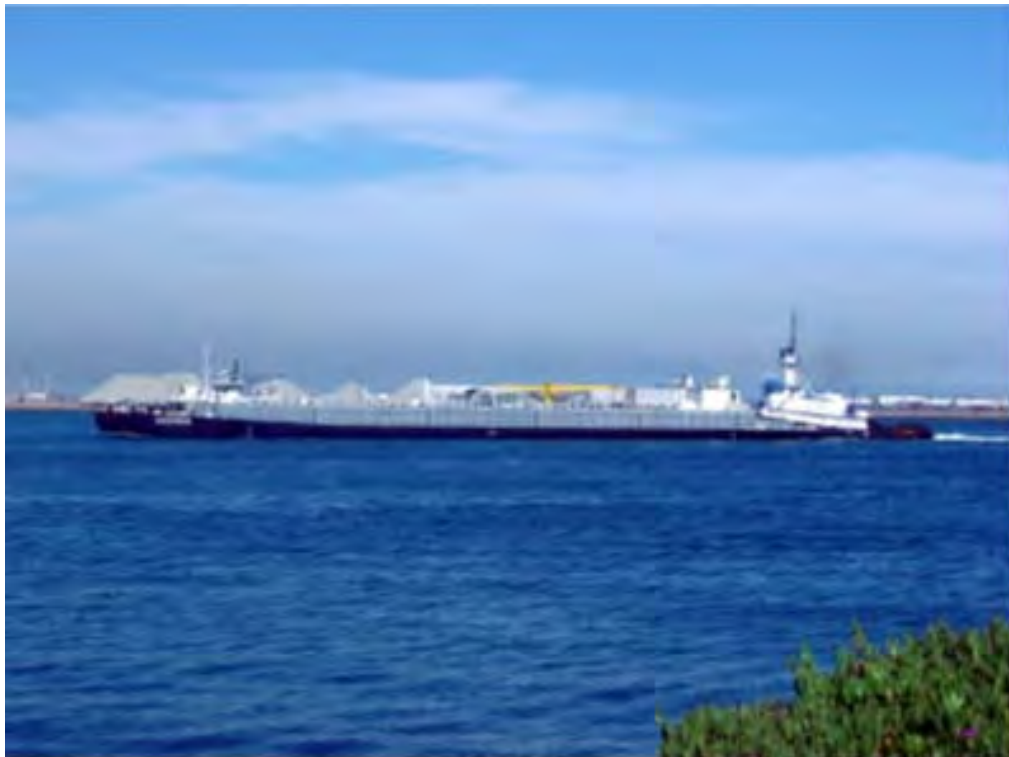
Figure 3.10: Integrated Tug and Barge
